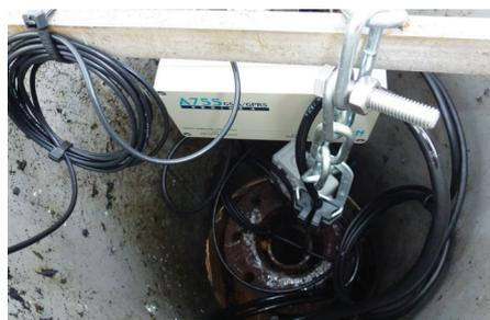
Envireau Water was appointed to develop an up-to-date monitoring network. After discussions and a site inspection, it was decided to install new, vented pressure transducers and telemetered data loggers to transmit data via the mobile phone network to the Envireau Data secure internet portal, where it is quality checked, processed and interpreted by Envireau Water's data management specialists. The equipment was installed with carefully positioned solar power
