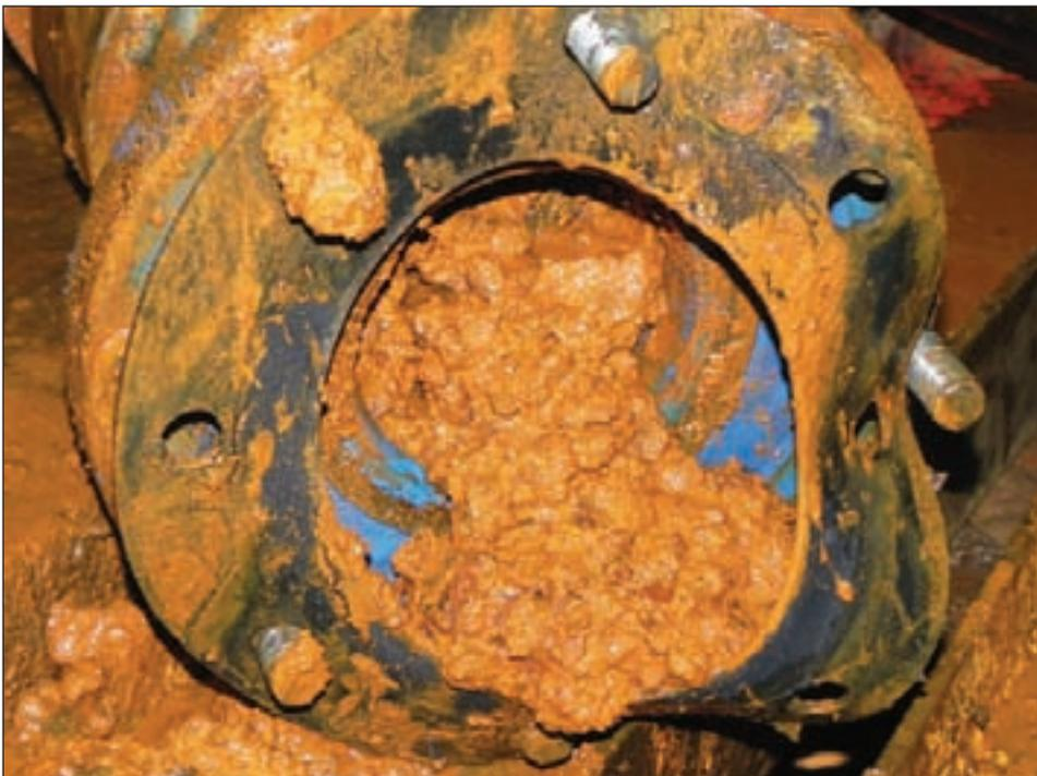
brates with atmospheric pressure, they precipitate. Biological activity reaction tests (BART) confirmed the presence of large colonies of iron-related bacteria that were proliferating in the borehole and resulting in the sludgy deposit.
