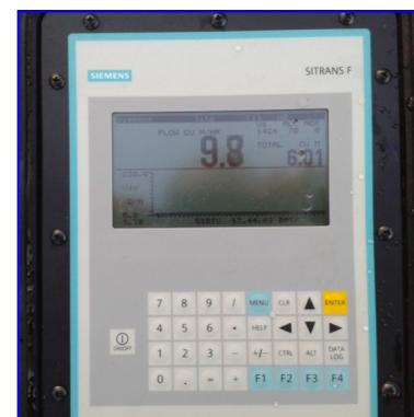
Following a successful verification exercise, if there are still concerns about the accuracy of metered volumes, then the type, age, condition and positioning of a flow meter should be considered as this can have a significant bearing on accuracy.
