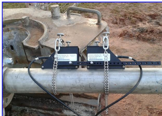
*A portable meter is strapped to the abstraction pipework to verify the installed meter*
