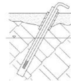
Inclined drilled well, crystalline aquifer
